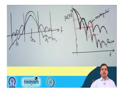
So, this particular rough sketch a compares the spectrum of the raised cosine and that of the rectangular, where it kind of depicts that raised cosine in a relative performance has a lower out of band. Although the main band is slightly wider, but finally, the out of band emission is lower compared to that of the raised cosine pulse shape.
