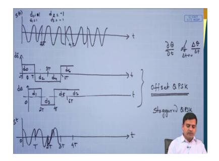
One could think of sending an offset; that means, a d 0 is for duration 2 T is for the entire duration 2 T and d 1 is also for the duration 2 T. So, in the unlike the previous case where both were for duration 2 T, but both were transiting at the same point in time, were is here what you can see is that, when one is changing the phase the other is remaining constant and when another one is changing phase the other one is remaining constant.
