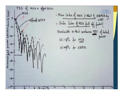
So, here what we have is the comparison with the MSK right and this is the one for the offset QPSK, whereas this is the one for MSK. Now the difference is that in MSK your
