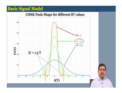
Now, this is the one, what we see for the GMSK. We had also discuss this and what we had pointed out is that for the for the BT value of 0.3, this is very critical value. And, it provide us good tradeoff between the band width and the pulse duration and helps us have a good shape which is used in the GSM modulation.
