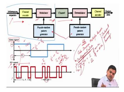
So, next what we look at is the third generation system, essentially the direct sequence spread spectrum, which is very much different compared to that used in the second generation system. So, we will take a brief look into how this things is structured and what is done and what is the advantage and how things are processed at the receiver? So, that we get to see the distinction between them. So, here what we see is that there is a data signal? Ok.
