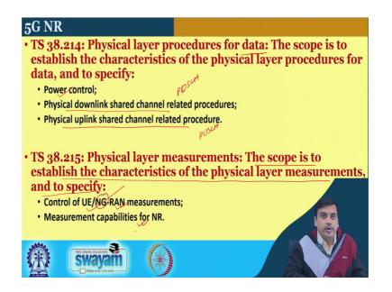
Then there is 214, which is with respect to the part of data. See the previous one is with respect to procedures for control, and physical layer control. Whereas, the next one is with respect to data right, and there also it is the power control, and physical downlink shared channel related procedures, so that is PDSCH and that one is PDCCH, PUCCH. So, here it is PUSCH, which we have described earlier ok.
