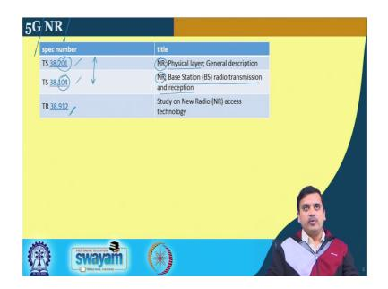
So, when we require the 38 series of documents, we are essentially talking about 5G from 3GPP perspective. And we are talking about NR or the New Radio from 3GPP perspectives. So, if one has to go into the details of these particular technology specifications, one would find 38 dot 201 which is the NR, again we are seeing that the name appearing often. It talks about the physical layer, so we have to go to 38 dot 201 document to get into the details as well as there are general descriptions.
