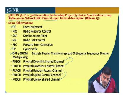
So, what we find is that the 201 document of 3GPP is the 3rd generation partnership project. It contains the technical specification of radio access network, NR, and the physical layer ok. And these are some of the abbreviations I do not need to go through all the abbreviations, you can easily understand them, and go through them as per necessary.
