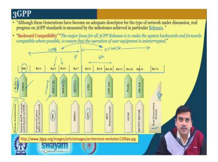
So, what we have here is basically two things. One is the radio side that means, the wireless signalling side. And the other is the system architecture ok, how the entire thing works. And this especially works with respect to the code network, the signalling, and the other aspects. And this one primarily talks about the wave forms, the air interface, and so on, radio access technology, radio access network.
