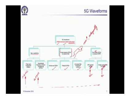
So, the different waveforms that were under consideration or that are still under consideration for the next generation are some forms of multi carrier, there are some form of multi carrier communication and they could be filtered there could be pre coded so various forms have evolved. So, what we find is that one set is coming under the pulse shaped OFDM.
