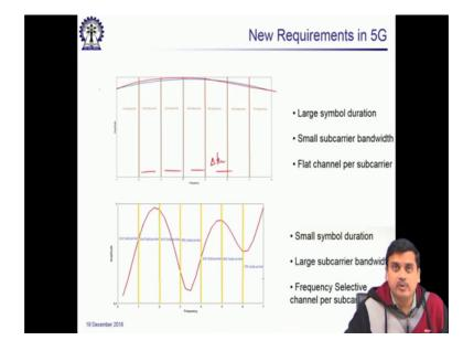
So, effectively it's boiled down to earlier more or less all the subcarrier so these were subcarrier spacing and the fluctuation was more or less flat across each of the sub carriers whereas, you have a situation like this and hence some solution is required to address this.
