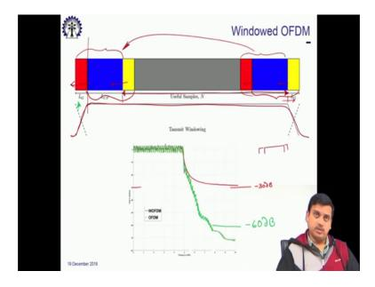
So, now, we take a look at the windowed OFDM architecture. So, in windowed OFDM this is the useful part. So, from here to here is the useful part of OFDM signal and there is a section which is copied as you can clearly see it is copied into the front. So, when it is copied into the front it is copied as the cyclic prefix, but then within that one would designate a guard section ok.
