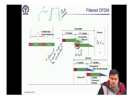
The next particular structure we can look at is a filtered OFDM so since we understand OFDM this is a this is not a very very huge modification from OFDM. So, in filtered OFDM instead of windowing one can use a filter impulse response to filter the OFDM. So, both can be thought of as kind of duels of each other.
