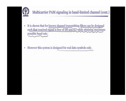
So, what we see over here or what we summarized is that it is shown that for known channel; that means, if the channel is known transmitting filters can be designed such that the received signal is free of ISI and ICI while attaining maximum possible baud rate signaling rate; however, the system is designed for real data symbols only right of course, you can change it for complex data symbols and what is one of the things that we are going to see next, in the next lecture.
