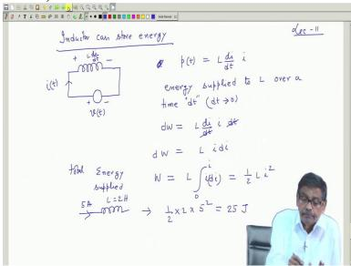
So we will see today that how inductor can store energy now, the thing is as I told you suppose you apply any voltage time varying voltage across an inductor + - Vt and then allow a current to suppose current at any time t i then what is the voltage across the inductance it will be this is + this is - I di dt is not. Now, if you look at the inductor, voltage across the inductor is L di dt with this polarity and current is entering through +.
