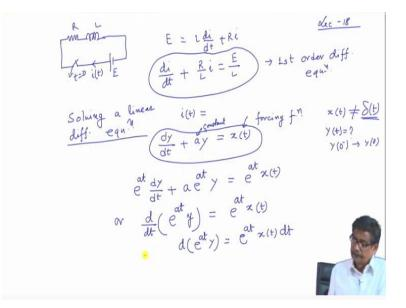
Now today what I will be doing is see while solving this circuit problems say RL.RC circuit discharging or charging circuit of both RL and RC type. Essentially what we are doing is we are writing down the differential equation and trying to solve that differential equation. Fortunately, the differential equations with constant value of RL and C will always give rise to a linear differential equation.
