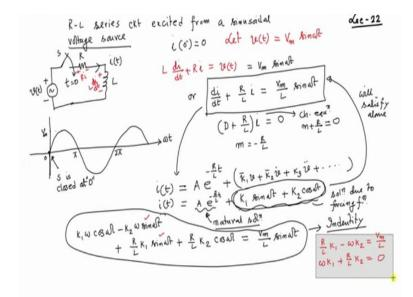
For example, consider a RL circuit; RL series circuit excited from a sinusoidal voltage source and so the thing is like this R here inductance in series L and here is a source which is time varying, vt is the voltage source and i0 minus this is the current I want to solve; i as the function of time and i0 minus is equal to 0, it is suppose given which was open for a long time and so on, now this switch s is closed at t equal to 0.
