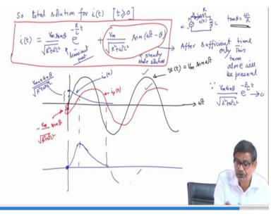
Therefore, total solution I will write in the next page as so, total solution for it, I mean I want to get the solution t greater than equal to 0 will be equal to it is equal to some e to the power minus R by L into t plus solution due to forcing function V max over this thing into sin omega t minus theta and here the value of the constant was found out to be this thing; V max by this into sin theta, so this constant is V max by root over R square plus omega square L square sin theta.
