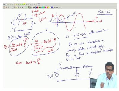
See, for example, we now know that we have seen suppose considered a simple analysis circuit series R and L, I told you that if you have connected a source which is suppose sinusoidal V st = V max sin omega t and I tell that this week is closed at t = 0 this equation. That means, if this is the supply voltage this is your V max or Vm I was writing Vm. So, if this is the supply voltage then and this axis is either time or omega t time t or omega t.
