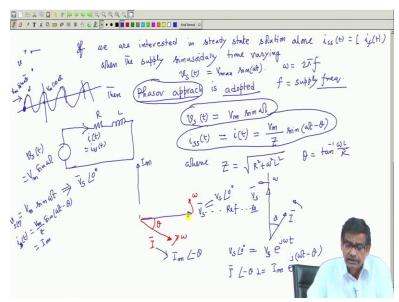
If we are interested in steady state solutions alone that is st which is ift forcing solution due to forcing function when the supply is that is a condition you cannot do for any supply for when the supplies finish sinusoidal time varying quantity like Vst is a Vmax sin omega t like that what is omega is 2 pi f, f is the supplying frequency. So, if we are interested in steady state solution alone when the supply is ready, then phasor approach is a adopted.
