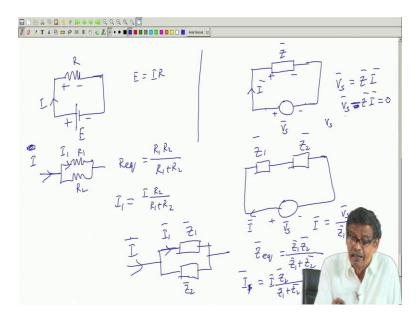
For example to impedances connected in series, just had them get the total impedance supply voltage divided by the total impedance will give you the current. Similarly to impedances are connected in parallel current in 1 branch I 1 will be total Current into get 2 divided by z 1 + z 2 and so on all the things that we learned in DC circuit will be applicable also here start Delta conversion of resistances connected can also be applied to start Delta calm conversion in impedances.
