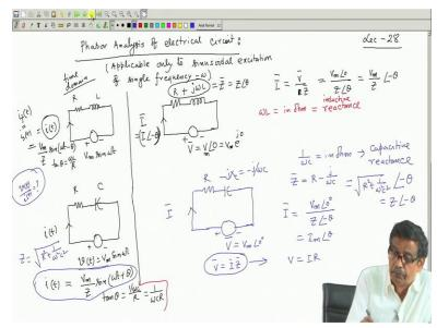
Welcome to lecture number 28. And as you know we have been discussing to analyze circuits using as a notations and in fact by further analysis, if you solve a circuit which is only applicable for excitation which is sinusoidal equation and the solution that you will get here will be the solution due to forcing function alone because transients will be born they will die after some time depending upon the time constant of the circuit how long it will last clumsy and that is decided.
