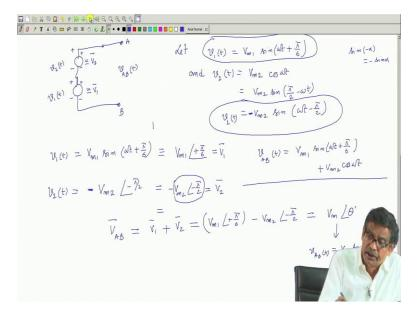
If I say giving you some example, suppose I say there are 2 voltage sources in time domain first time doing it is given as V 1t and another sources which is with the polarities are important mind you, this is V 2t and both are sinusoidal and this is A, this is B. So, suppose let V 1t V is equal to V maximum 1 sine omega t + Phi by 6 suppose, somebody says sinusoidal voltage And V 2t to somebody says V 2t is Vm to its maximum voltage into cause omega t.
