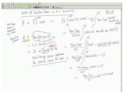
So, active power is denoted by generally capital which is average power average power absorbed by the load by load. So, this average is generally it is average I even if I did not write it means average capital P and it was shown to be equal to be V RMS into I RMS into cosine theta is called average power then reactive power that is this really this is nothing but essentially over a full cycle vt it d omega t 0 to 2 phi. This is the average over a cycle.
