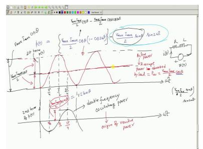
That is what you must understand because you see, you recall that average power origin of reactive power V max I max by 2 quickly now after knowing RMS value I know it is VI sin theta and what it is it is the peak value this peak value of the double frequency oscillating. So, the physical significance of VI sin theta is also about the oscillating powered and the peak of that what is the real power like the power it is the average value of p high you must understand that.
