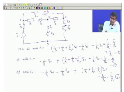
Similarly, nodal analysis let me just write down the equations no question of that deriving it. Suppose, you have a circuit like this am now drawing impedances as boxes suppose 0 1 bar is 1 voltage source. There is another impedance here and there is another volt source is here and AC there is Z3, Z2 to this is a Z3 they could be RL or pure a combination of art and capacitance and so on.
