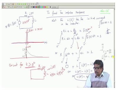
So, our lecture number is 35 and in this lecture I will tell you now we have made enough ground to find out the response say for example in RL circuit when it is excited with an impulse voltage x t or V t = delta t, this voltage source vt = delta t. We even need him an unit impulse function in the laboratory you cannot get that sinusoidal square wave does that you get but in it impulsive cannot get, but the important is will show later that if the circuit is linear and time invariant.
