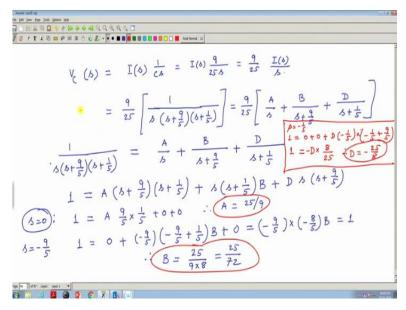
So I will say now I am interested to know capacitor voltage. So I will say capacitor voltage will be vcs will be nothing but Is into 1/cs now 1/cs c value is 4/25 capacitance value c value was so much 25/9 c value so I will say Is into 1/25/9 so it will be 9/25 into s which = 9/25 into Is/s then you put already I have calculated Is that = 9/25 will be there Is was s + 9/5 into s + 1/5 and there is 1/s another so this will be vcs here also I have to expand it to partial fraction.
