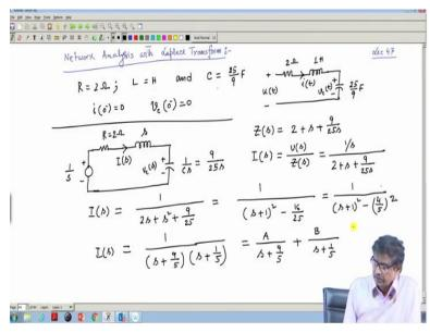
Welcome to 47th lecture and we have been discussing with the network analysis using Laplace transformation and if you remember our circuit will be in time domain with RLC values provided. Then next step will be to replace this redraw the circuit in each domain replacing R/R by R that is no replacement for our resistance replace l/sL and replace any capacitance by 1/cs and if you assume that the initial conditions are relaxed that is all the capacitor voltages are 0 initially.
