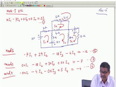
Easily see suppose you have a network like this I will put some numbers said, this is 3 ohm, this is 4 ohm This is 7 ohm this is suppose + -10 volt, this is + -12 volt and this is another resistance said 18 ohms and here is another branch which is 12 ohm and here is a voltage, 7 volt and here is another branch where is a voltage there say 1 ohm and this is a + -4 volt suppose this is the network all the currents are to be found out.
