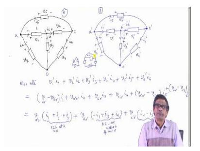
Similarly I could do which is just few lines I will write because it is necessary also this is network B this is network A also node that v1 dash into i1 (()) (27:25) + v20 dash voltages of this networks multiplied by the respective current in the first network that is network A actual current i2 + v3 dash + i3 + v4 dash i4 + v5 dash i5 + v6 dash i6 what this comes out to be. Okay same procedure v1 dash is what voltage across this element in terms of the node voltages v dash a0 - v dash b0.
