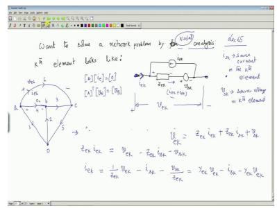
Welcome to 65th lecture on network analysis and we have seen that how graph analysis can be utilized to solve a network problem completely by using the loop analysis method. Similarly we can solve the net or same Network problem by nodal analysis. So, we started with this you recall that this is the general element and this is the thing and this portion I will just delete and straight away write that this is the basic equation which will be this one.
