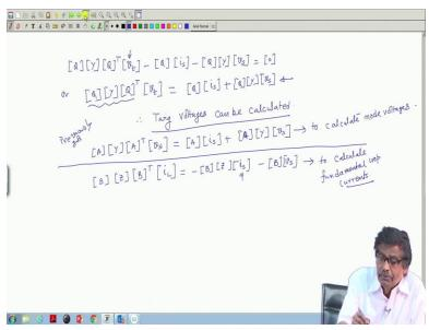
So, this is thing and this is equal to zero or I can say that my target is to compute this one so Q into y into Q transpose into vt will be then equal to Q into is + Q into y into vs that is all. So, this is once again the nodal admittance matrix here we got Ay transpose when we apply nodal
