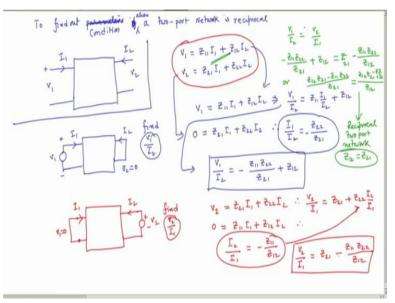
For example, that is I will write it like this; to find out parameters, if a 2 port network is reciprocal, I will better write to find out conditions, when a 2 port network is reciprocal, that way it is better to express. So, let us take with respect to z parameter, suppose this is the network, this is your V1 and this is your; first I draw the raw 2 port network this is how it is, in general these are the things.
