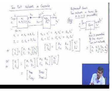
Two port networks in cascade. In cascade means the output of one port is the input; the output whatever you get from the first port is connected, suppose this network 1 it is plus minus V1, this is I1 you connect it and here another network into whose input you connect to this port, get the point. This is plus minus; this is V2. And say, so V1 it will have its terminal and you consider this to be your V1 dash.
