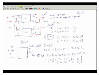
This is lecture 77. So we discussing about series connections. Similarly, if you can connect this one in parallel also. For example, if you have a two port network like this, this is suppose V1 and this is I1 and this suppose V2 and this is suppose I2 these are two port networks okay. Now here another network which are having things like this. This is plus, minus V1 dash, this is plus minus V2 dash and this I1 dash and this is I2 dash, this is the thing. Okay.
