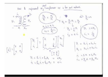
Suppose, how to represent a transformer and ideal transformer as a two port network. We know what a transformer is. Suppose we have a ideal transformer here. These are the dot terminals of the transformer. Ideal transformer means no resistance, no linkage flux etcetera. And if you apply a voltage here we will get some induced voltage there, this is number of trans N1, this is number of trans N2, and if it delivers a current I2 in this direction.
