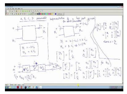
Parameter representation of a two port network, two port gyrator, I want to do it. So the thing is like this. This is + -V1. This is i1, but here I had assumed it to be i2 to be this way. And we got this relationship that is V1 = -k i2 and V2 = k i1 and this is too V1 = -k i2 and V2 = k i1 that is the thing, usual thing. But if I want to represent it in terms of what is called the A, B, C, D parameters you know what we do is this, this direction of the current of i2 is to be reversed.
