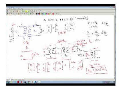
So this is the transformer and; we say that in terms of A, B, C, D parameters or sometimes called T parameters transmission lane parameters. It will be that is the transmission lane parameters means V1 i1 should be there that is the input voltage and current is represented in terms of output voltage and current that is V2 i2 and this we got a 0 and this we got 0 1 / 8 because V1 = V2 and i1 = i2 / a, ideal transformer. a is N1 / N2. That is fine. This is the thing.
