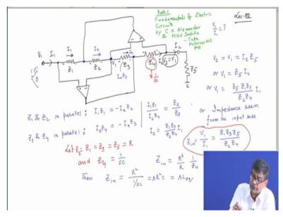
Let us first draw the circuit without much words, so that you will be able to understand what I am doing. For example you take 4 impedances, although I am drawing resistances it is true for any impedance say, z1 here, this is another impedance I could also draw a box but anyway, z2. Suppose, there are 4 impedances you connect, z3 and you have z4, very interesting circuit z4.
