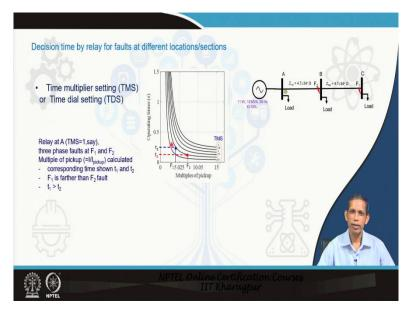
A decision time relay for faults at different locations and sections, see here, time multiplier setting for this one characteristic, let us say this is inverse definite minimum characteristics. So, these are different curves, they are having different time multiplier settings, this one TMS here, if you multiplied 0.5, then we are getting this curve, we multiply with 3 then you are getting the uppermost curve and like that.
