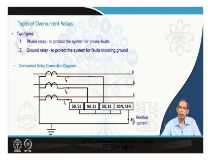
Now, how these corresponding relays are? Overcurrent relays in one perspective can be divided into two, we call them a phase relay and ground relay. Phase relay takes care the phase faults like ab fault, abc fault that is 3-phase fault and ground relay takes care of all faults involving grounds like phase a to ground phase b to ground and so. So, these are the two types of overcurrent relays that are used in system protection perspective for different elements.
