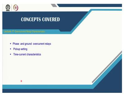
So, the coverage in this lecture will be on phase and ground overcurrent relays, then we will go to this how to select pickup setting, and the required time-current characteristics for a particular protection scheme. (Refer Slide Time: 1:06)
