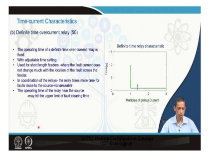
Next, we will see the definite time overcurrent relay. So, here we see again designated by same number. In the definite time overcurrent relay, we see a characteristics we have some definite time delay here, fixed time. However, these definite time delay can be changed as far the wish of the relay setting engineer to have the corresponding requirement.
