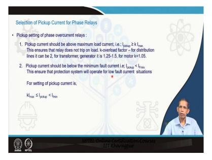
And continuing, now we will see this pickup current above which the relay takes a decision is very critical in the relay design perspective. Now, how the pickup currents for the 2 types of relays: phase and ground relays are being selected that we will have to see. So, first you can see that for phase relays selection of pickup current.
