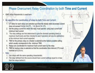
Now, we will go to the better approach of doing this. Phase overcurrent relay coordination by both time and current. So, we have seen individually current and time and now we will see how we can combine them for a better coordination. So, we have seen the limitations of both also. Current, its limitations if the feeder length is small then it has a problem and time the problem is that more time it requires when it goes towards the source relay.
