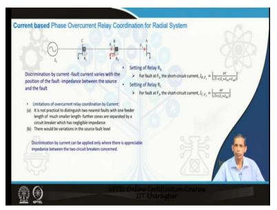
Let us first come to the current based phase overcurrent relay coordination for radial system. This is radial system. Source or the substation in this side and then we have, you can see that 3 buses and they are feeding to different loads. So, this is the current base, the discrimination is achieved by only the current magnitude.
