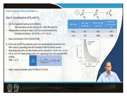
Now moving forward, now we will go with the coordination with  $R_C$ . So how we will coordinate that current? This 965 A current which are seen by these, at that time the relay  $R_C$  also will see 965 A of current but relay C has CT ratio of 150:5, a factor 30. Relay will see 30.17 A in the secondary side.
