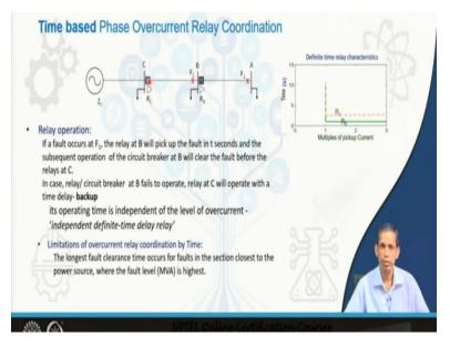
The other option is time based phase overcurrent relay coordination. Here, we are talking about the time is the basis not the current. So, we have already seen earlier different characteristics for overcurrent relay and one of them it is nothing but definite time relay characteristics. So, we talk about definite time for this, any current more than the pickup current, relay trip immediately and that you can say that the corresponding setting is adjustable in this case.
