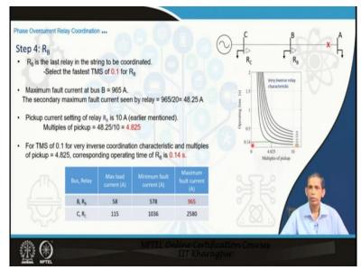
Now, we will see what is the corresponding  $R_B$  relay characteristics and the corresponding for the  $R_C$  relay. First the  $R_B$  relay.  $R_B$  relay is the guiding factor. Select is the fastest TMS that is in the set of curves. The lowest curve is the 0.1 so select this curve for the relay at  $R_B$ . Now, the maximum fault current for bus B at this point is 965 A. This relay that is your maximum fault current for  $R_B$  is 965 A.
