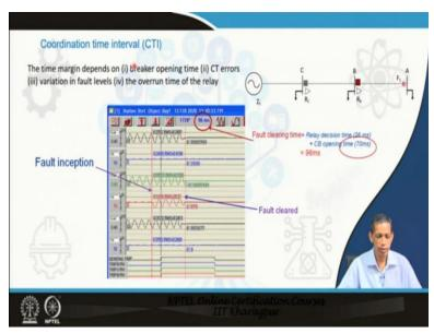
Now, we talk about coordination time interval that happens to be 0.2 to 0.4 s, 10 cycles to 20 cycles for a 50 Hz system. These depends upon a number of factors. Important are breaker opening time. The breaker opens see the relay commands, let us say the fault is at F<sub>1</sub>, the relay picks up, commands the breaker and the breaker opens. Fault is clear so this section is out. This load and the rest of the system remains intact. That is what is being expected.
