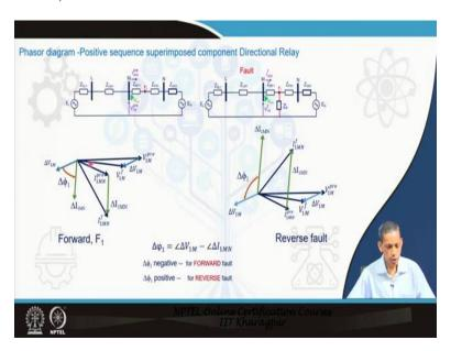
Now going to the phasor diagrams like we did for the sequence component also so we have prefault and we have fault sequence diagram, positive sequence diagram. Now let us first go for the forward fault like what we have seen here. So, we have  $V_{1M}^{pre}$ , we have  $V_{1M}^{F}$  so this is  $\Delta V_{1M}$ . We have current
