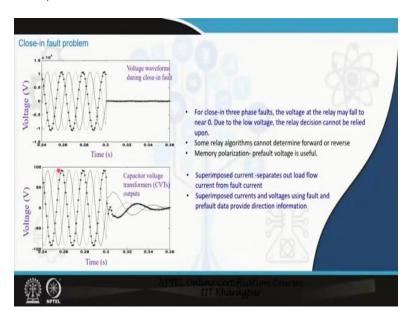
Moving further let us first appreciate an issue. Now suppose, in a system we have already explained that a fault happens to be closed to the relay bus, in that case all the voltages  $V_a$ ,  $V_b$ ,  $V_c$  will collapse if the fault happens to be a voltage three phase fault. Once again if the fault is close to the relay bus and happens to be a voltage three phase type then all the voltages will collapse simultaneously.
