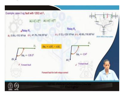
Now if you see this performance of the  $R_1$  you got the delta Phi 1 to be negative, negative even though the fault resistance is very high, it is correct. And the  $\Delta \phi_1$  minus 114 degree is  $R_2$  that is also correct. So, we consider that both the relay correctly identifies the direction of fault using the principle of superimposition quantities. And so we see that the corresponding superimposed
