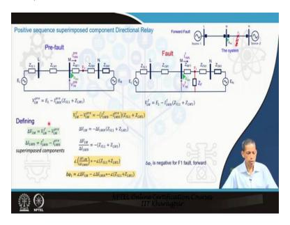
Now we will go to how the superimposed component can be advantageous for directional principle. So we will use positive sequence superimposed component. As already mentioned superimpose component, superimpose current is that the fault current minus the prefault current that gives us you can say that the corresponding superimpose component. Let us consider this system.
