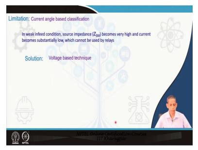
But there are limitations to this current based classifications. In case of weak infeed, when the source impedance becomes very high the current magnitude become substantially low and that leads to, the phasors computed by the relay not reliable, and therefore, we may not able to use the corresponding angle correspondingly. Then what is the solution? The solution is can we use the voltage information? Yes.
