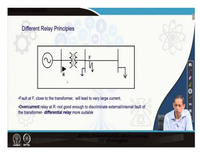
The other things that, see this circuit here, we have a transformer connecting to a source or substation and we have a line section. This fault happens to be closed to the transformer and we have relay protecting the transformer at R, then the relay using only the over current principle may not be able to distinguish whether the fault is in the inside the transformer or beyond the transformer.
