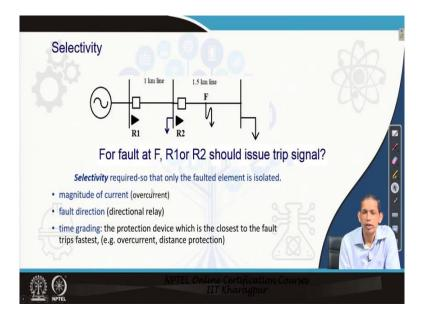
Now, on other aspects of protection scheme, let us see this circuit, substation source, we have two sections or line. And let us say that a fault happens to be at point F. Now, in this case, there is a clear mandate here that the relay should make a decision and trip the breaker so that this section can be isolated and the rest of the portions including this load can be made from this substation.
