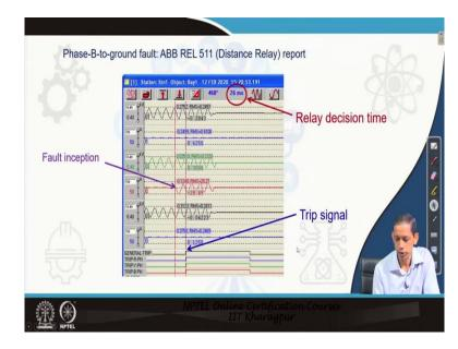
Now come to an example, on this aspect, so in a system there is a phase-B-to-ground fault and a relay that is numerical relay records the event. See in this case  $U_1$ ,  $U_2$  and  $U_3$  are the voltages for the RYB phases, where  $I_1$ ,  $I_2$ ,  $I_3$  are the corresponding currents. Now if you see the plots corresponding to  $I_1$ ,  $I_2$  and  $I_3$ , phase B current suddenly jumps up to a very high magnitude, this means that this is the inception of the fault and the fault continues.
