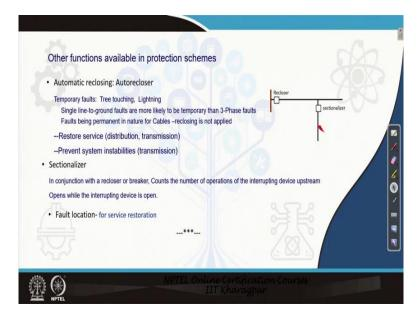
The other functions which are available in protection schemes, like you see here in this example we have a fault in this lateral and then we have a recloser arrangement. Now what the recloser does is that because in an overhead line most of the faults are transitory in nature they remain for some time and they vanish.
