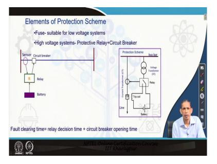
So, we know the usage of fuse that we use in our house wiring also so whenever there is a fault or a short circuit in the circuit, then the current becomes high and the fuse is blown out. So, in that case the faulted part becomes isolated from the rest and the rest of the circuit remains intact. Repair the faulted portion and then replace the fuse that circuit also can be restored.
