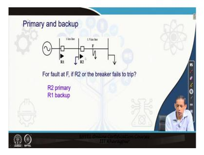
Now see this network, source or substation, feeding to two line sections and a fault in the second line. In this case R2 relay should actuate the breaker, and let us think of a situation when the relay R2 fails, or the breaker fails to open, or the communication between R2 and the breaker or the battery you can say that supply fails at this point. That means that the fault will continue and that will lead to damage in the system and issue that life security and so.
