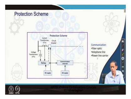
Going more into this protection scheme, we have breaker, we have the relay actuated by the DC supply we have sensors voltage transformers and the current transformers. In addition to that, today numerical relays are having a facility to communicate the information to other relays or any substation devices or they can also receive information from other relays also to have a better decision making for the protection.
