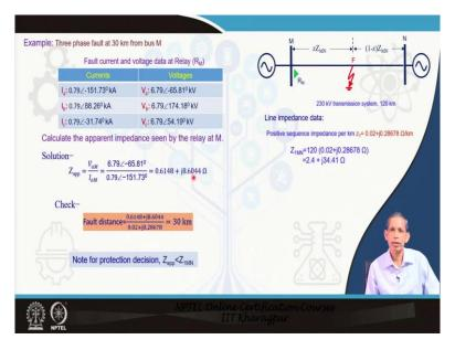
Now, we will go to an example for such a system, 230 kV, system 120 kilometre line length, and we have the positive sequence impedance per kilometre small  $z_{1=}$  (0.02 + j0.28678)  $\Omega$  per kilometre. So, this is nothing but from the resistance and the corresponding inductance of the line available. So therefore, the corresponding total positive sequence impedance of the line  $Z_{1MN}$ , Z is 120 × per kilometre impedance. So, that gives us Z = (2.4 + j34.41)  $\Omega$ .
