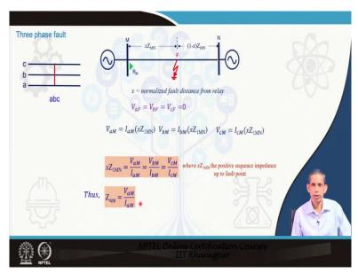
So, let us see for different types of fault, how the apparent impedance calculation will be related. 3-phase fault, balanced, so we have 3-phase fault. So, let us say this is the 2-bus system. We have a transmission line between M and N's buses, and our distance relay is at R<sub>M</sub>. We
