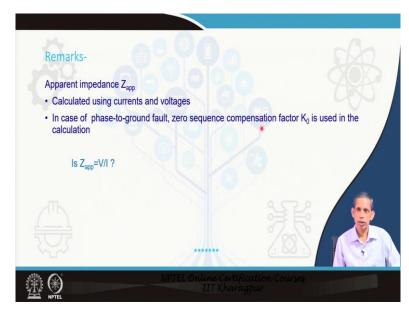
So, in summary, Z apparent calculation is integral part of this distance relay. It uses the local currents and voltage for this. For that, the corresponding relation, proper relation of the Z apparent will require a fault classification, fault type must be known. In case of phase to ground fault, 0 sequence compensation factor is being used only for only for phase to ground fault, not for any other types of fault.  $K_0$  happens to be complex also and depends on the line parameters.
