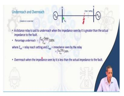
Now before going to that let us be clear on two terms, the underreach and overreach of a relay. So, what we see let us consider this transmission system and we have relay at the bus M. So, consider distance relay in zone fault at F. So, it is inside the zone 1. Now if the relay now finds the apparent impedance to be greater than the actual fault impedance, positive sequence fault impedance then we call we consider this situation as underreach.
