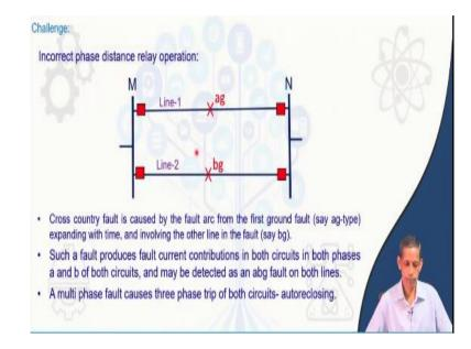
Another challenge is the cross country fault so what do you mean is that suppose line 1 as you can say that phasor-to-ground fault and associated with this arcing and so. A fault may be triggered in the other line or circuit in another phase like here in this case we have shown phase b-to-ground. So, what will happen that both we consider distance relay at this point and this point or from the other side also in the network that they will see significant current in phase A and phase B.
