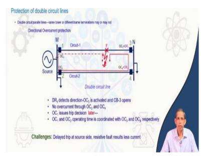
Now let us we will consider a simple double circuit system however, double circuit or otherwise called also parallel lines can be can run on same tower, can be running on different towers and the same nearby right up way they can be terminated at different nodes, they can have a common bus also and the other bus may not be common. So, there can be different configurations on double circuit line in a power system.
