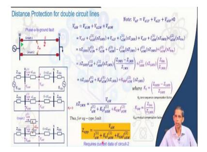
So, this leads to our analysis for double circuit line little bit different then what we have derived the apparent impedance calculation for single circuit analysis. Now, let us consider the double circuit line here phase a-to-ground fault we have analyzed for other fault also similarly you can analyze fault in circuit 1 and we have a zero sequence mutual impedance between these two lines  $Z_{0m}$ .
