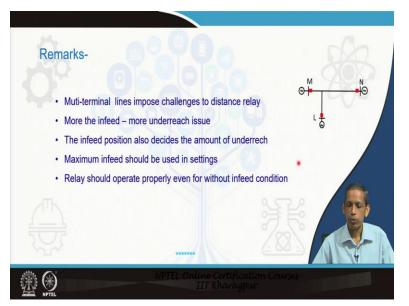
So in overall, we see that multi-terminal lines is a challenge for protection, particularly, for distances relay we saw here even through examples also. More infeed, more under reach, further the position of this infeed is also a factor in the amount of under reach issue, particularly for zone-1, of course, zone-2 and zone-3 also have also under reach issue.
