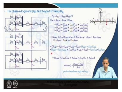
Now we will see for the same system, same fault point, we will see now the what happens for the phase a to ground fault, its analysis. We know for phase a to ground fault, the fault point voltage  $V_{aF} = V_{a1F} + V_{a2F} + V_{a0F} = 0$ . Now, we see here, this V<sub>aM</sub>, the relay bus voltage during the line to ground fault will be available from this calculation related to this sequence component analysis.
