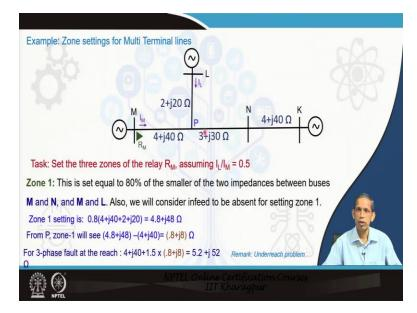
Now, we will go for the zone-3 setting for the system. In zone-3 setting, similar to the zone-2, what you do is that the apparent impedance of the M-N, M-N infeed is (4 + j40) + (1.53 + j30) up to this N section. So, this impedance plus considering the infeed (1.53 + j30) for zone-3 also we will go for the higher length distance. So, this becomes  $(8.5 + j85) \Omega$ .
