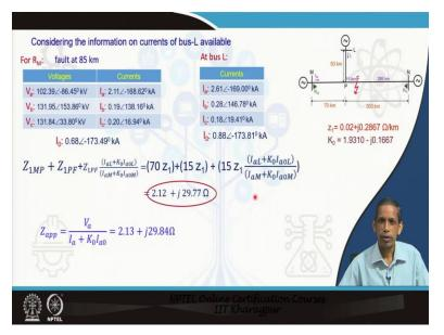
Now, we will see that the apparent impedance which you have derived for the phase a to ground fault, that is, that can be validated if you know the corresponding bus L, the infeed currents which we have noted here. 3 phases current at bus L, during that same fault corresponding zero sequence component of current. So, we have already derived these for the phase a to ground fault;
