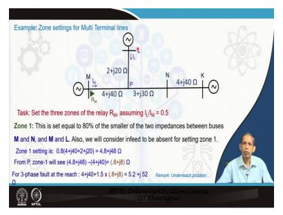
So now, we will go, you can see that guidelines are being applied for transmission system having multi terminals configuration. So, we have considered a system like this, the corresponding T point or the tap point it is P, one section here, the infeed section from L to P, and then the another section from P to N. Now for zone-3, we have considered another exam from N to K in an interconnected power system. But we see here, you can see that this is a multi-terminal line and so, from N also,
