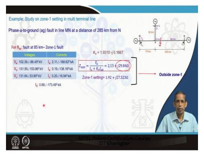
Now, we will see for a phase a to ground fault in the system the corresponding zone-1 is good enough or not. For this, in this system, if phase a to ground fault created at 85 kilometer from bus M which happens to be in zone-1, as you have seen this setting, the zone-1 covers physical distance of 96 kilometer. So, therefore, this fault at F, which is only 15 kilometers from P, this part is 70 kilometer, happens to be in zone-1 fault for  $R_M$ .
