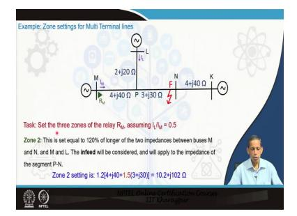
Now, next, we will go for consider the zone-2 setting. The zone-2 setting is 120 % or so. We know the two-terminal line of longer of the two impedances, in this case, multi-terminal line, it will be 120 percent of the longer the two impedances between buses, M and N, and M and L. So, we have from this relay bus, we will have two sections 1 and 2, and the other one you can see that is the, this one. So, whichever is the longer out of that, 120 % with the consideration of the infeed.
