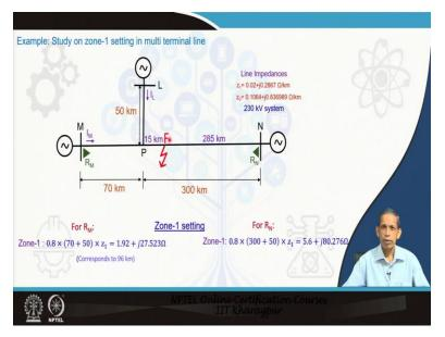
Now we will take a case example, simulated example how the zone-1 performs in a multi-terminal line. In a 230 kV system, we have considered the way we have done a 3-terminal line. So, it has a 50 kilometer here, 70 kilometer this section, and we have a 300-kilometer long line from P to N section. The 0-sequence and the positive sequence per kilometer impedances are available to us. Now we will see how the zone-1 setting will be there and then we will assess how good is the zone-1 setting.
