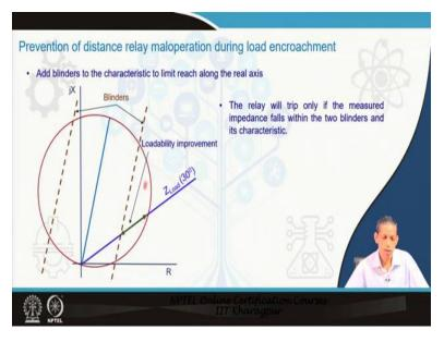
Another option, add blinders to the characteristics to limit reach along the real axis. So as I said this is the portion for the load so what will be that? Suppose this is a mho relay characteristic also, you put two blinders the dotted lines blinders. These are parallel lines with the load line. The transmission line impedance line, line impedance line, this is impedance line and it parallel with that.
