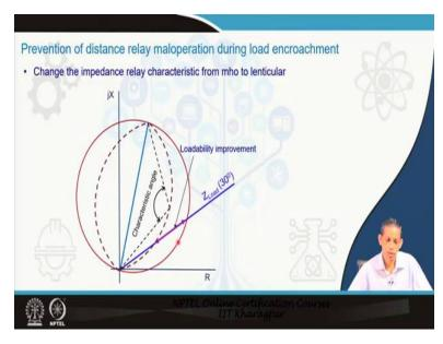
Then what is the solution in this to overcome the corresponding load encroachment in longer lines or heavily loaded condition and so. We will discuss few methods that is being those are being used. First one, Change the impedance relay characteristic from mho to lenticular. If a line is having is expected to be that load encroachment issue so what to do that the corresponding characteristics, say zone-3 characteristics.
