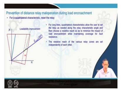
The other one is a quadrilateral characteristic setting. So what we see here that in these kind of situations, if we expect to the cover the RF for you can say that let us say zone-3 relay having this. But if the corresponding relay characteristic is expected to be load encroachment issue, so we reduce the coverage, you reduce the coverage and thereby we can say that, we can exploit the advantage of this portion as the improvement portion.
