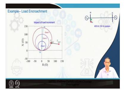
That reduction in apparent impedance is of concern now. Will it enter to the relay characteristics? Then the relay may malfunction. Take a situation of 400kV line here and the Z apparent was at a particular instant was having at this condition.
