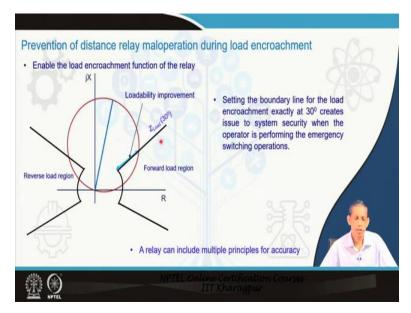
The other one option is that the enabling the load enforcement function. So we have a special characteristic for this load perspective. So typically you can set these two lines 30 degree, 30 degree but and then you can say that in both the sides forward region and the reverse region, this we consider the load. So therefore we can say that in the mho characteristics also, this portion we can say that will be not allowed to we can say that trip.
