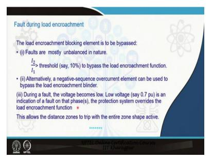
Now take another issue. If a fault happens to be there during a load encroachment period, try to understand the apparent impedance seen by the relay is in the load encroachment area and at that time the relay is blocked because it should not trip. And if fault happens to be there in that zone, because this is a fault so the relay must trip, the relay is to take care.
