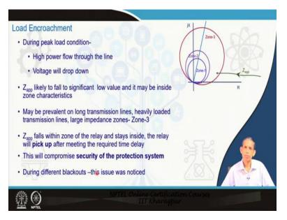
So we say that the load encroaches into the characteristics, the Zapparent seen enters into the relay characteristics during loading condition, particularly heavily loading condition then that creates unnecessary tripping security issue.
