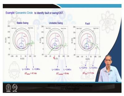
What the relay does now, for these 3 cases that this is stable swing case first case using the voltage and current we obtained the corresponding  $Z_{app}$  and V/I for any phase and then we have the concentric circles here the outer and inner. So, when it goes to the enters, so, that touches the outer circle, then the time recording starts and then only touches the inner circle the time recording stops.
