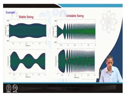
So, this is the situation of stable swing voltage and current patterns and the unstable swing the corresponding voltage and current pattern this is clearly visible as the distinction.
