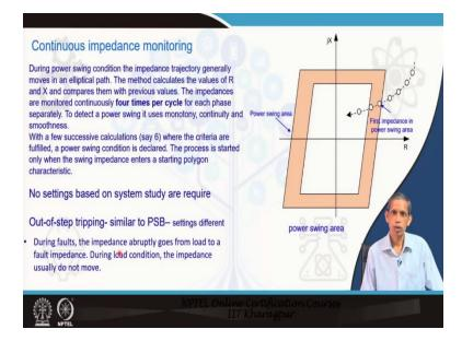
For that what is being done a a power swing area is being assigned like we talk about concentric circles and so, and once it starts entering to that the process of against that the corresponding impedance calculations the 3 tests against that what to mention in the earlier slide are starts beginning and then the relay you can say dot the said calculations 4 times per circle circle or circle per 50 Hz systems you can assume 5 milliseconds kind of thing.
