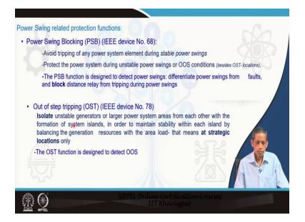
So, as mentioned, we have solutions for power swing issues. One perspective on power system Power Swing Blocking (PSB) device number 68 in IEEE device number. Now this is to avert unwanted tripping during stable power swing. The PSB function is designed to detect power swings, its objective is to distinguish swing from faults.
