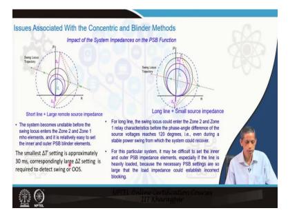
Now, some of the issues also with the Concentric Blinder Concentric or Blinders both are manner similar perspective. So, what do you see that when the corresponding trajectory traverses like this, then the angle goes on increasing. Now, let us see the situation short line large remote source impedance. Line is short. So, this impedance is small and large remote source impedance and the source impedance locally.
