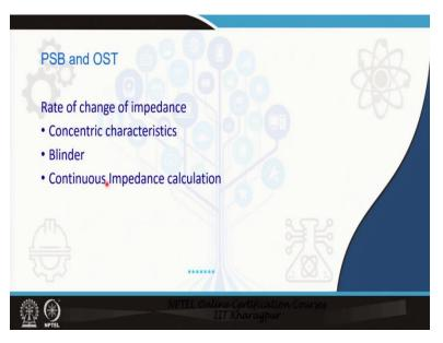
So, in this lecture, we mentioned about power swing blocking and out of step tripping and we address on the three techniques based on rate of change of impedance principle, the concentric characteristics, the blinder and the continuous impedance calculation, the merit of the continuous impedance calculation why is that being used. So, in many relays, you can see that in numerical relays, that advantage, it does not depend upon any system, a system stability study.
