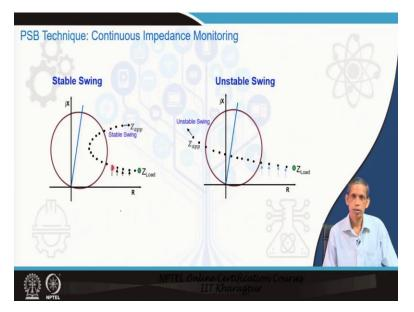
Now, to go to the third technique in this impedance calculation perspective continuous impedance monitoring. So, what is being done here that the apparent impedance traverses like this. So, we go on monitoring considering the corresponding apparent impedance and then we can start to require some calculation. So, in case of a stable swing it traversal like this.
