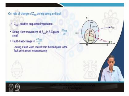
Now, coming to different techniques on rate of change of impedance. So, the impedance we wish to talk about in the distance relay, the  $Z_{app}$  which is being calculated or seen by the relay is the positive sequence impedance and that refers to the positive sequence impedance up to the fault point. If it is a fault, that is what we have learned.
