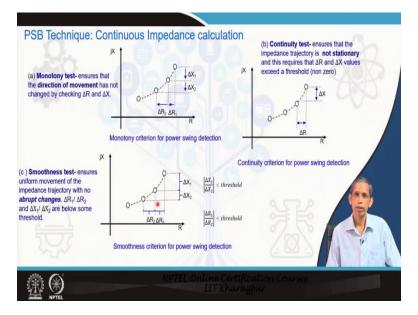
What has been done here that the continuous impedance calculations as already mentioned, 3 things are being checked Monotony test, Continuity test and Smoothness test, these 3 tests are being checked by the relay and from these 3 it then confirms whether to swing or a fault. In monetary test, what is being done there to the direction a moment has not changed, you can see that has not changed that is being checked from  $\Delta R$  and  $\Delta X$ .
