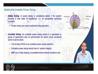
In the last class, we are discussing on how power swing creates problem to distance relay. There we saw that the impedance trajectory during swing enters into different zones and that may lead to unwanted tripping in the distance relay. So, distance relay is vulnerable in this case during power swing. Then how to overcome it? The solution for that will be discussed in this lecture.
