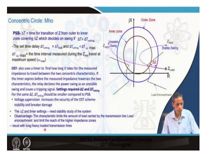
Now, more details on this. So, what we say that the PSB function passes pass power swing blocking function. So, we have  $\Delta T$  time of transition of Z from outer to the inner covering, so  $\Delta T$  the measurement. So, when the apparent impedance traverses this kind of path during swing, so, this is our  $\Delta Z$  the impedance difference between these which are fixed for this setting.
