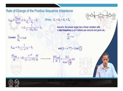
Now, let us analyze what this Rate of Change of Impedance reveals. So, we have a two bus system as usual and a current flowing from left to right from bus M to N. So, this is swing situation we are talking about, not a Fault situation.  $Z_{app} = \frac{V_{Relay}}{I_{Relay}} = Z_T \frac{E_S}{E_S - E_R} - Z_S = Z_T \frac{1}{1 - (E_R/E_S)} - Z_S$  where  $Z_T = Z_S + Z_L + Z_R$ . So, that we have seen in our earlier discussion in last lecture.
