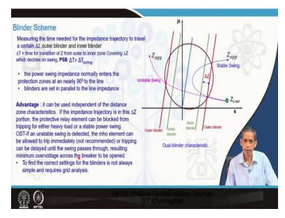
The second method is on Blinder Scheme similar to that one based on same principle of dZ/ dt and so, what is being done here here we can say that blinders outer blinders, inner blinder and to this sides also inner blinder and outer blinder. So, here also what you do that this is your  $\Delta Z$ . So, these blinders are generally parallel to the line impedance and they can be positioned not necessarily outside that is the advantage of this approach.
