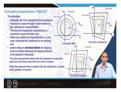
Now, they we will different techniques based on that we learned from the last slide that dZ/dt for the distance relay is indicative to distinguish fault to power swing. Now, how that is being used in different techniques we will learn so, first one is concentric characteristics. So, what is being done here, if you see the mho characteristics here, so, this is a zone which is of concern the point is that these zone needs to be protected from power swing.
