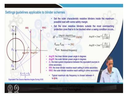
Now, some of the guidelines for applications to blinder schemes is that if you can see that this is about resistance reach outer and the inner what we have discuss. Suppose a blinder is here and if you see the total impedance of the system source, remote side, local side and this is the line in if you see that from this here suppose here the traversing point you can say operates at here and the way we discuss in the earlier also.
