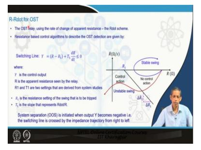
The R-Rdot approach is used for out of step tripping specific utility only. So we know that when the apparent impedance becomes smaller than a value, then the distance relay should go for a trip decision. So with that philosophy that if the Z is smaller than X value, then the relay will trip.
