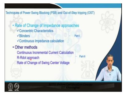
So in the last lecture, we discussed about three techniques based on the rate of change of impedance; the concentric characteristics, blinders, and continuous impedance calculation. We discussed what both power system blocking and out-of-step tripping and we demonstrated examples on stable swing, unstable swing, and fault; how the relay is able to distinguish them.
