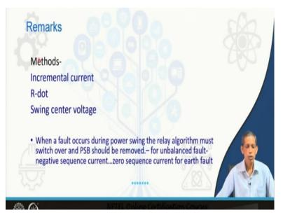
So in general, we saw in this lecture 3 methods. Incremental current, only from the current signal; the R-dot approach to have out of step tripping business; and then finally, swing center voltage approach and its derivative we talked. The derivative gives information on that whether it is to distinguish swing from fault and whether it is a stable swing and unstable swing in supplement with the swing center voltage decides.
