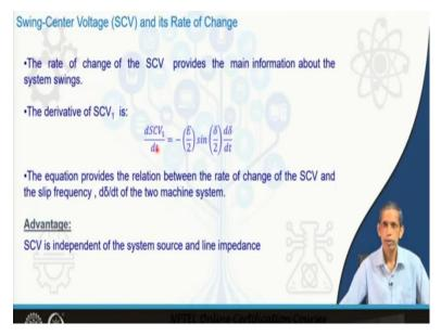
What we will do now that with that swing center voltage SCV1 if we take the derivative of that one,  $\frac{dSCV_1}{dt} = -\left(\frac{E}{2}\right) sin\left(\frac{\delta}{2}\right) \frac{d\delta}{dt}$ . So this shows that the derivative of the swing center voltage is having only in terms of the  $\delta$  terms and the voltage. The equation provides the relation between the rate of change of swing center voltage and the slip frequency  $d\delta/dt$  for the two-machine equivalent system.
