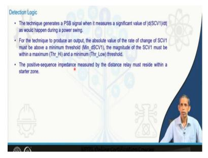
The technique generates the blocking signal, power swing blocking signal when it measures a significant value of swing center voltage say, derivative dSCV1/dt. D $\delta$ /dt, I am saying that from that one if you calculate the corresponding dSCV1/dt then we will find that it will be very significant one power swing.
