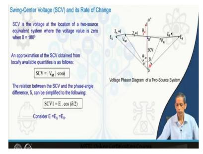
Now, I will move forward. In our earlier discussion also, we have this kind of diagram on the impedance. Now, to this impedance, if we multiply I, then we get the voltage. So then this becomes also the voltages. So this is source voltage  $E_S$ , this is  $V_M$  and this is  $Z_SI$ , the  $Z_LI$ , and this  $Z_RI$ . And this straight line, as we have discussed earlier, is nothing but the total impedance of the line, so ZI, you can say the dotted line.
