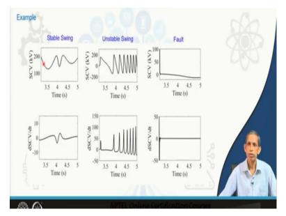
Now you see that the swing center voltage, how do you compute this? V  $\cos \varphi$ . We have this V measurement at the end bus, at the local bus, relay bus, and the corresponding  $\varphi$  angle between voltage and current. So that V<sub>M</sub>  $\cos \varphi$  gives us a swing center voltage. So we have plotted this one for this swing center.
