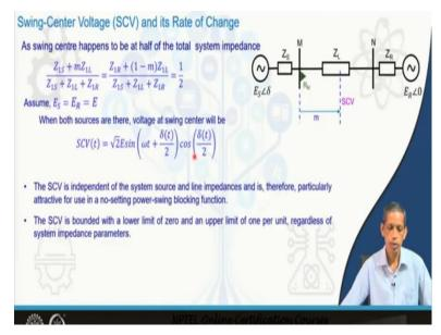
Now, what we see, that we know earlier also that this location is half of from both the sides. The swing center or electric center is half of the total impedance of the line,  $Z_S + Z_L + Z_R$ . So that gives us that these 2 impedances which we are looking from this side or that side what we have calculated in the earlier slide,  $\frac{Z_{1S}+mZ_{1L}}{Z_{1S}+Z_{1L}+Z_{1R}} = \frac{Z_{1R}+(1-m)Z_{1L}}{Z_{1S}+Z_{1L}+Z_{1R}} = \frac{1}{2}$  because it points to that point only.
