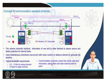
So, how the communication system can be useful and that may enhance the you can say that the performance of the distance relay we like to see that in this slide. So, have these relay at M bus and we have the relay and the distance relay set at N bus. Now, let us say you consider here assuming a communication medium is available and, and what you see here, let us you can say fault happens to be here in this line towards the bus N.
