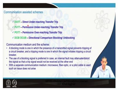
They are important you can say that 5 we can say that basic communication assistant skills which are being used for high voltage system with their distance relay schemes, DUTT direct under reaching transfer trip, PUTT permissive under reaching transfer trip, and POTT permissive overreaching transfer trip, and directional compression blocking and unblocking it is DCB and DCUB.
