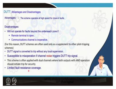
The advantages you can say that of this direct under reach transfer trip scheme is that the schemes operate very fast for the close-in faults. And it also clear you can see from the other end also but it has associated disadvantages, it will not operate for faults beyond the under reach zone. If it means that if the corresponding fault from M bus side as you have seen earlier.
