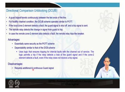
The last one on directional comparison unblocking. So, earlier we were talking about blocking, now it is unblocking, agree? So, unblocking means you can say that it is a trip kind of thing. What has been done here? A guard signal travels continuously between the 2 ends. What we have learned in DCB, that only a block signal is being issued from the remote terminal you can say that reverse third zone relay to have a secure decision when the fault happens to be the beyond the line.
