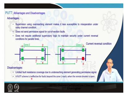
The PUTT has advantages the supervision using overreaching element makes it less susceptible to misoperations, even to the noisy signal channels also, agree. Because at the AND operation does not stand you can say permissive signal for out of section faults. So, that say that AND operation advantages does not require additional supervisory look to maintain security under current reversal condition for parallel lines.
