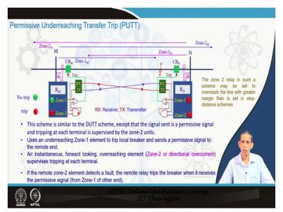
We will go to the second 1 the permissive under reaching transfer trip, permissive. So, with permission only you can say that the remote end will operate, it is not like the direct under reaching transfer trip and under reaching transfer trip. So, the word under reaching means again the zone 1 is the information platform which is PUTT transfer, which has to be transferred to the other end.
