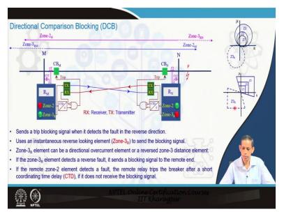
Now, we will go you can say that to the, the other you can say that scheme. Directional comparison blocking, DCB. Now you have your blocking signal not tripping signal. So, in our earlier cases, only tripping signals for being transfer whether it is underreaching from the or it is being from the overreaching means zone 2 or so. Now here you can say that we have directional comparison.
