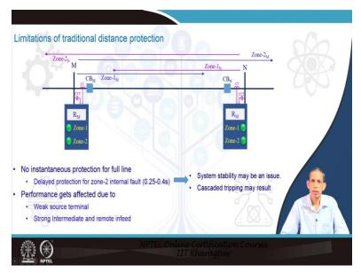
Now, let us see the issues with the traditional distance protection. So, we know we can say that, in an interconnected system a set of relays that to the bus M and another set of relays at bus N will be there to activate the circuit breaker as N, when required. So, here we have sown zone 1 from this side and zone 1 and zone 2 from M side and also zone 1 and zone 2 from this side.
