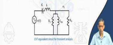
Now, we will go to the transient performance of this CVT. So, we saw that during normal steady state it is expected that the voltage which is there in the primary proportionate voltage in phase voltage will be available to the secondary that is to the relay, but during transient what is the situation that we like to analyze. Steady state error for this CVT is pretty negligible for protection application.
