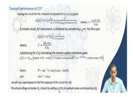
Now solving the circuit for the, transient component of  $e_2$  i.e.  $e_2(s)$  gives
