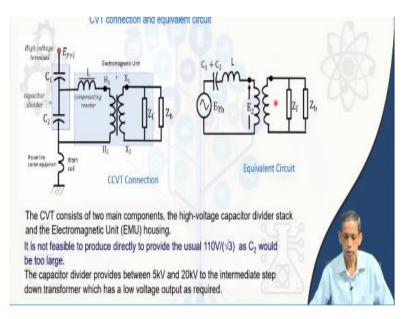
Now, to see how this CVT functions what are these different components of CVT. First, we will discuss on the steady state perspective and then we will go for the transient analysis situation like fault or so. A CVT as already mentioned is a capacitive voltage divider so it has a stack of capacitors. This part is connected to the bus or to the conductor as required. So, this is the high voltage terminal this red point here.
