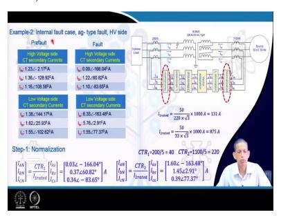
Next case we will go for an internal fault case, so same arrangement for the transformer, only the corresponding fault is created in between the two sensors, group of sensors CT and you have created a fault internal to this arrangement. So, it is in zone fault in this case. For this case the prefault condition remaining same for this both high voltage and low voltage side.
