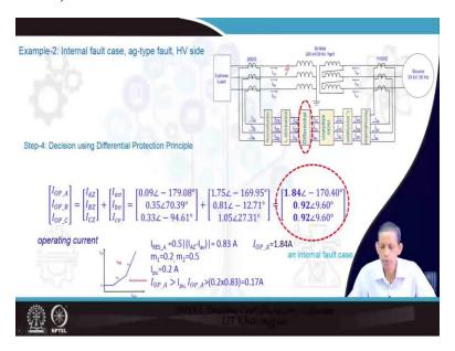
Now, final step is on the decision making process, so for the operating current for each phase of A, B and C we get the corresponding this plus this and then we add these two current phase or
