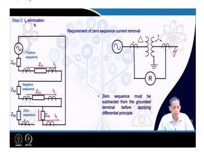
Second step is on I<sub>0</sub> elimination, so a zero-sequence eliminations. Let us first see why we require this. Now, this is a simple system, a transformer fed from an AC source, three phase transformer of course, this side is delta, this is star, star grounded and so. So, we have CT this side and CT this side and this is the differential relay which does the calculation for operating current, restraining current and make a decision perspective analysis.
