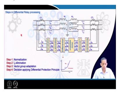
In overall the differential relay processing, the differential current processing the corresponding characteristic which we talk about here for calculating the operating current and the restraining current and to make a judgment whether the operating current above the corresponding characteristic or not. This judgment is obtained through different steps of the processing of the currents available from the CT.
