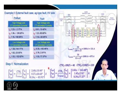
We will go to examples, how the corresponding steps are being accomplished and then how the differential relay can make a judgment whether the fault is external or internal. First we have considered for an external fault, ag-type fault in high voltage side. So, a simple system we have considered, a 33 kV source grade and then we have a transformer, the transformer is 220:33 kV and then the transformer is Ygd1 and 50 MVA transformer.
