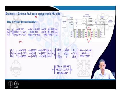
Now, for this external fault we will go for this step three, that is the vector group adaptation, the phase angle coincidence perspective and so. So, we have the corresponding matrix, k equals to 1 here because this is a Yd1 connection, so substituted value of k then you got the corresponding angles to be cos30, cos 150, cos(-90) and so then this rotating kind of thing.
