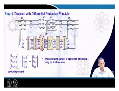
Now, the final step is on decision with the differential principle, so we already got vector group adaptation then from this side we have already zero-sequence elimination perspective, this is low voltage side, this is high voltage side and then the middle one is about the differential current is to be calculated and the corresponding differential characteristic principle has to be applied.
