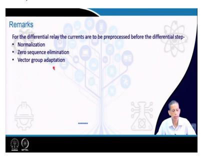
So, we see that the differential relay essentially requires four steps and all four steps are important. The normalization of the current has to be carried out, the zero-sequence elimination to subtract the corresponding zero-sequence current is also required and then to have the corresponding phase shift carried out by different vector groups that are to be carried by the vector group adaptation.
