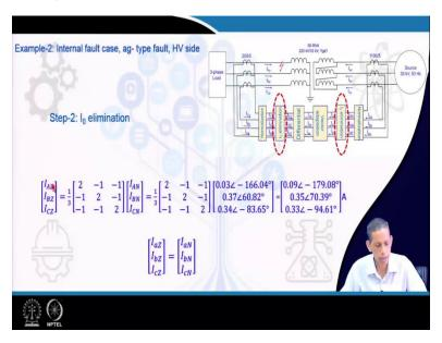
Zero-sequence eliminations  $I_{AZ}$ ,  $I_{BZ}$  and  $I_{CZ}$  capital and then a small  $I_{aZ}$ ,  $I_{bZ}$ ,  $I_{cZ}$  the way we did for the earlier case of external fault case multiply this matrix and got the corresponding currents to be 0.09, 0.35, 0.33 for the high voltage side. And then the same is for the low voltage side the  $I_{aN}$ ,  $I_{bN}$  and  $I_{cN}$ .
