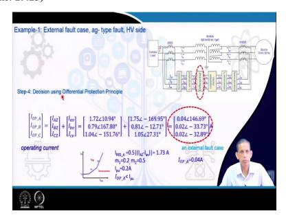
The fourth step is on the decision process, the differential current calculation and the restraining current and then applying the corresponding trips. So, we got the corresponding operating current to be
