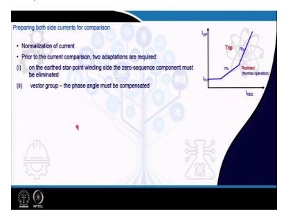
Now, in the last lectures, we have seen that differential relay is a promising technique for transformer protection. But it needs proper processing of the current like the normalization aspect before the corresponding differential of high voltage winding side current and the corresponding low voltage side winding current are being analyzed.
