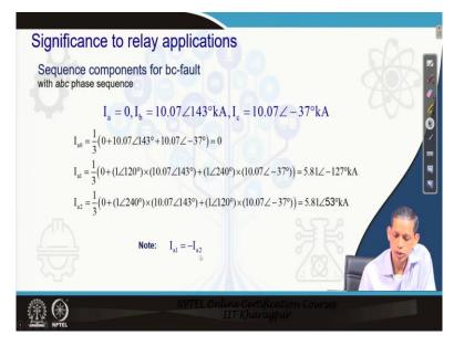
The other case, see here  $I_b = 10.07 \angle 143^0$  and,  $I_c = 10.07 \angle -37^0$  and if you analyze you can see that  $I_a$  current is no more, fault is involved with only phase *b* and *c*. So, we see here, in this case
