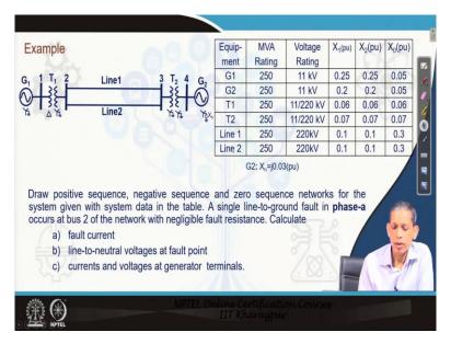
Let us consider one example, here. So, this is a system where we have two sources here connected by, double circuit transmission line, circuit 1 and circuit 2 and then they are connected by a transformer,  $T_1$  and  $T_2$  and the  $T_1$  here is connected into delta ( $\Delta$ ) to the generator side and star ground (Yg) to the line side and the right hand side  $T_2$  is connected in star grounded- start grounded (Yg-Yg) to both the sides, you can see that in this case.
