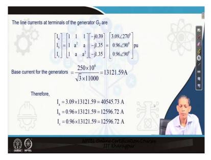
So therefore, the line current terminal from the generator 2, can be find out from the sequence components multiply by T matrix,
