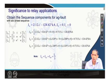
Now for the line to ground fault case; phase *a* only is involved with the fault,  $I_a$  is only there,  $I_b$  and  $I_c$  are 0 and by analyzing this what you get,  $I_{a0}$ ,  $I_{b0}$ ,  $I_{c0}$  all are having the same magnitude and angle. So, the relation for this is
