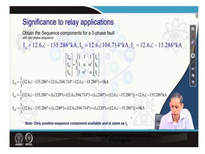
Let us analyze, this system for a case, see here this phase *a*, phase *b* and phase *c* values are given to us. So, obtain the sequence components for the 3 - $\phi$  fault. This is a 3- $\phi$  fault as I<sub>a</sub>, I<sub>b</sub>, I<sub>c</sub> magnitudes are same and they are 120<sup>0</sup> apart. Now, it is concluded that if we calculate the sequence components using
