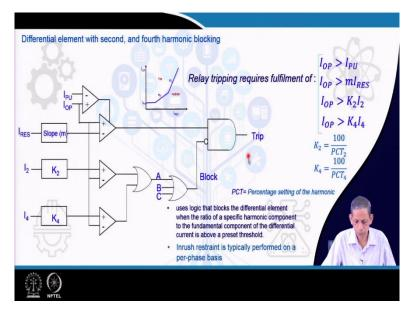
Now, come to first, these harmonic blocking scheme perspectives. So, this is what conventional percentage differential relay. To trip, the corresponding fulfilment requirement differential will operate, it means that it confirms an internal fault when these conditions are being satisfied. This we have already known that the I<sub>OP</sub> current, that the differential current in the part, in the, in that part, in that algorithms, which we have seen earlier in earlier lectures also.
