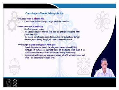
So now, to distinguish, Overvoltage versus Overexcitation Protection and note, I am saying that we need not confuse about this perspective. This is a differential relay protections we are talking about. differential relay protection should operate only when an internal fault happens to be the transformer and that case is neither the inrush situation or the corresponding overexcitation situation.
