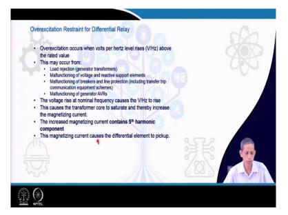
One thing we see, that the Overexcitation restraint for differential relay, the operation of course, when the volts per hertz of the rated value, this may occur from their load rejection, malfunctioning of voltage and reactive power support, the voltage high situation. This increment of flux in the core that leads to the large amount of current in the magnetizing part.
