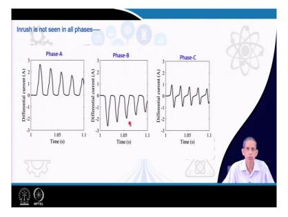
This inrush has various other issues that you see here. That whenever inrush happens to be there, all the phases, they are being switched on; this is a three-phase situation. So, all are through the different polls. In a circular curve they will be switched on. It is being observed that all the phases do not see large current due to this inrush situation.
