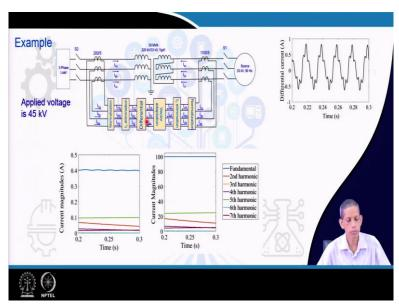
Then, when you analyse, the corresponding current magnitudes of different harmonic components and in terms of the percentage of the fundamental also, then decide that corresponding the fifth harmonic component, the green one, each of very high value and which will make the corresponding, the blocking arrangement for the differential relay operations.
