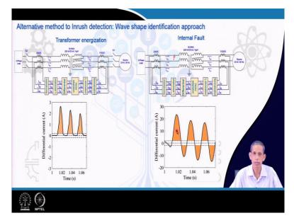
The alternative method also to the, this inrush detection process besides this harmonic-based approach and so, one is called waves shape identification approach. Let us see for this case. So, transform energizations and internal fault. So, these were the internal fault case and this normal transform energization. So, in the transform energization, we have the inrush shape like this or to the negative or a very small amount.
