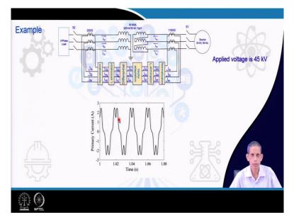
So, for example, in these, the 33: 20 kV systems, we apply 45 kV equals to these 33 kV side systems and the corresponding signal nature becomes this, which is having highly third harmonic component, also fifth harmonic component, but as already mentioned, the third harmonic component will be eliminated by the zero sequence component eliminations. So, the differential current will be availing only only significant amount of fifth harmonic component.
