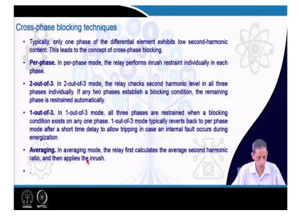
There are different solutions that are called cross-phase blocking techniques for the inrush situation. Now, the blocking options we have already learned, but how that is being accomplished in a three-phase environment that we like to figure out here. The cross-phase word is similar to the cross polarization that we learn in the differential relay perspective, that in the directional relay perspective.
