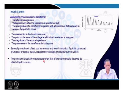
This inrush current, what we you say has the issue associated with unnecessary tripping. This current is not only do transformer energization, it occurs also when there is voltage recovery after the clearance of an external fault. The energization of a transformer in parallel, the
