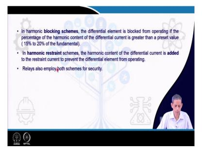
In the harmonic blocking, schemes for inrush situations, there are 2 schemes, one is blocking scheme and the other is a harmonic restraint schemes. Well we can learn what these two also in our subsequent discussion here. In the blocking scheme, typically when the second harmonic components become greater than 15 % or so with respect to the fundamental.
