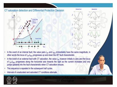
Now, let us go to we applying these concept for and IOP versus IRES plane, that what you see that the corresponding if this dotted line is a  $45^{\circ}$  line for this plane, then as already enumerated that the  $i_{OP}$  and  $i_{RES}$  increase simultaneously for internal fault the for internal fault the situation will be that or difference cycles of operation the corresponding operating point will be around this dotted line.
