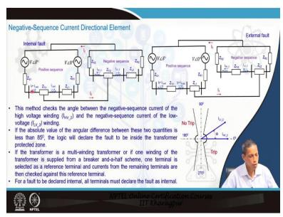
Then another approach the negative sequence based approach and that is based on directional principle. Now, how this principle is there just have a look on this. So, we have the same system and same unbalanced situation of these for not involving ground and we have positive sequence diagram negative sequence diagram and so these for internal fault for external fault positive sequence diagram and negative sequence diagram.
