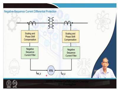
So, in overall such a negative sequence phase you consider a scheme can be summarized to like this from CT signals from the three phases will scale scaling phase shifting both the sides zero sequence eliminations and all these things whatever you carry out. In addition to that will extract the negative sequence current from the low voltage side and from the high voltage side and this negative sequence currents will be now coming for the comparison perspective.
