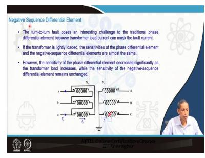
Now, coming to how we can apply other principles in the differential relay also so many manufacturer also provide in differential principle the negative sequence differential element and there being use full in this special cases and in some cases they are very sensitive also like to see how that can be applied and how these negative sequence-based differential principle can be useful. Let us, assume a transformer where we have only faults across few turns.
