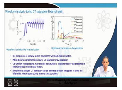
So, how to overcome this issue? So, we will analyse the corresponding current and then we will try to find the solution mechanism to address the CT saturation issue for external fault case. So, we see that the corresponding differential current pattern as in the earlier slide for external fault case you find a pattern like this and if we analyse the corresponding current in terms of the different harmonic components then it shows the patterns that the harmonic currents to be like this.
