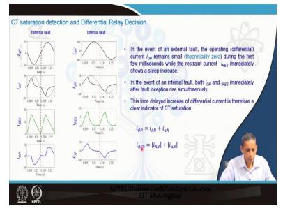
Now, let us move further details. How we can detect CT saturation for the differential relay decision process. So, we have two situation external fault and internal fault what we have already
