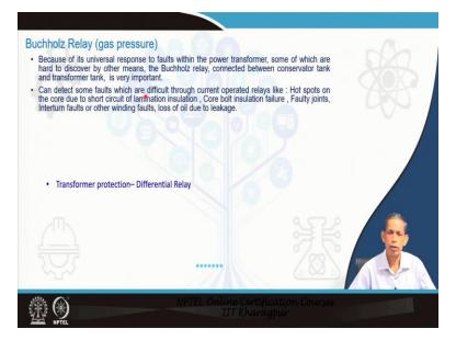
In addition to the electrical signal based principle for transformer protections especially differential relay applications and so. There are other gas relays and so particularly Buchholz relay is of significance which it takes the position between the conservator tank at the transformed tank and whenever some incipient fault or minor fault happens to be there.
