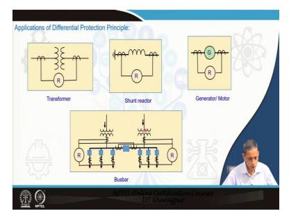
We learned the differential protection for transformer how to connect the CT in star grounded and star side and star side star connections and how to have to we have to ground with both the sides and how to process the corresponding signal for successful applications we learnt also transformer differential protections how to apply negative sequence base approach restricted earth fall how to have the corresponding CT saturation issue also
