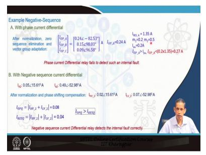
Now, what happens that given the data sets what you have say after the normalizations zero sequence elimination vector group adaptation. So, the corresponding phase A, phase B, phase C currents are there and the fault in phases so therefore associated current in phase A is more and we expect that this would go for the trip business for the phase based relay so we say that  $I_{OP_A}$  is 0.24 that we are taking now  $I_{RES}$  during that time for phase A is 1.35.
