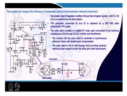
Now, will have a test systems, we were going to different network protection schemes. So, this is 39-bus New England systems. We have some modification here to integrate the corresponding renewable resource, 345 kV 60 Hz at bus number 33, here we replaced the corresponding a synchronous generator by PV plant with the inverter into interface and with adding to transformer perspective. The inverter with this solar plant is controlled in
