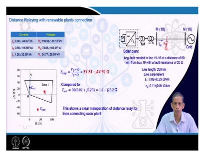
Now, we will see a third example on distance relaying with renewables. So, for the same system, equivalent system of the 39 bus system seal line number 19-16. So, we created fault at 80 km from the bus 19 with the fault resistance of 20  $\Omega$ . And the fault type is *cg* fault type. So, what we see here is that the line length is 200 km and line parameters are positive sequence, same as negative sequence, and zero-sequence provided here.
