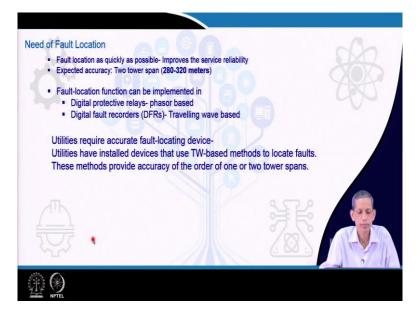
Utilities required quick assessment on the fault position of a transmission line, it has reliability issue, the sooner the line is restored, better we can manage the system. A line may be dealing with thousands of MW, so deficiency in one area may create problem. It has associated revenue loss and also service to the loads and customers.
