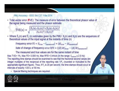
Now, we have seen that the corresponding PMU provides not only phasors, also provide frequency and rate of change of frequency and we are concerned about more accuracy here. So, the PMU accuracy follows certain standard, IEEE standard IEEE Std.C37.118a-2014 governs the level of accuracy the PMU must have. Particularly on the protection application perspective.
