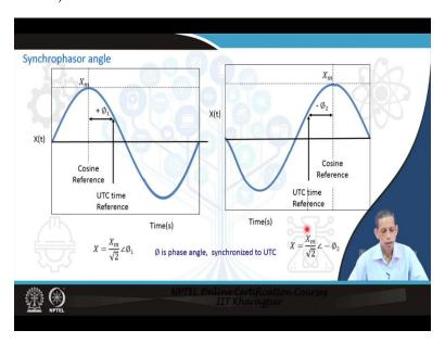
How the angle is being estimated? Otherwise that will lead to improper angle reference and it becomes purposeless application. So, we have this corresponding sinusoidal waveform, now we have the cosine reference having a positive peak in this cycle this UTC time reference as already mentioned this is through by the device measuring PMU relay or so which has the GPS antenna.
