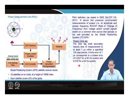
For the phasor measurement unit PMU, this is a device and it is being conceptualized from the relaying area and it has gone to many other areas of applications in power system particularly on monitoring and control application also. So, PMU is a just like a numerical relay kind of thing, so it has analog inputs, anti-aliasing filters to avoid the interference of high frequency components. Then A to D conversion process. So, this analog to digital gives us this samples as you know.
