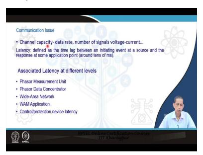
The communication issue is the most challenging things here as it requires dedicated communication systems on the PMU and the wide area measurement system perspective. The channel capacity of the communication system depends upon as you know data rate that is the number of voltage current signals, what are to be passed to that communication and to how many PMUs or PDC perspective so that will decide the channel capacity.
