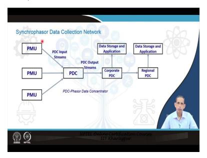
In the synchrophasor or the synchronized data which are being provided by this PMUs in the systems and they are to be collected to have meaningful applications of those data. So, from different PMUs the phasor data concentrator collects at the substation level or at zonal level, the corresponding *n* number of PMU data are being collected, collated and integrated. Again, it is being send to the different next level of PDC like, corporate PDC, regional PDC level.
