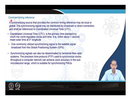
So, what is that common time reference which can be achieved in a power system application perspective? A synchronizing source that provides the common timing reference may be local or global. The synchronizing signal may be distributed by broadcast or by direct connection in terms of fiber optic cable or so and shall be reference to coordinated universal time, UTC time.
