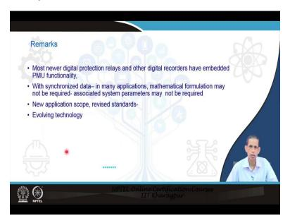
So, in overall we see that the phasor measurement unit which provides time synchronized data or called synchrophasor. Protection or control applications becomes viable with that kind of time synchronized data which has also the time information, with each phasor.
