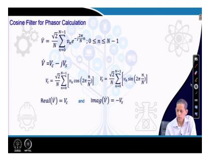
Now I will go to another category of filter extension of the one cycle DFT with term mention is that cosine filter and then again for the phasor calculation aspect. So, let us see that how this cosine filter uses for phasor calculation and then we will see through example how we can obtain the corresponding phasors for different windows of a signal.
