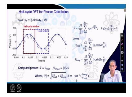
Now I will go to more, further more efficient way of doing things for the Phasor calculation using the concept of discrete Fourier transform, the next one is on half cycle DFT, so we see here same signal let us say
