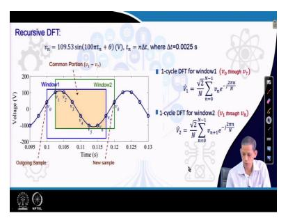
So, we proceed with this one cycle DFT the corresponding first window phasor, this window where the corresponding window samples are  $v_0$  through  $v_7$  and then the corresponding equation becomes
