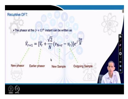
So, in general we can conclude that at any instant  $(r + 1)^{th}$  instant that any phasor can be obtained from the just earlier phasor computed at the r<sup>th</sup> instance written as
