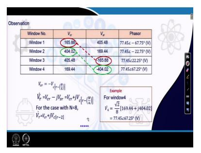
So, in overall we can conclude that window 1, window 2, window 3, window 4, four windows we have computed and we have computed the corresponding  $V_{cr}$  and  $V_{sr}$  the cosine part and the sin part for the corresponding window, we got the value to be what we obtained these values are noted and the corresponding phasor values are noted down here. So, what we derived in the cosine filter perspective is that
