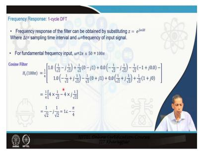
Moving forward, we see what you do with that, for the frequency response of the filters you bring that z transform the cosine and sine filters, if you substitute
