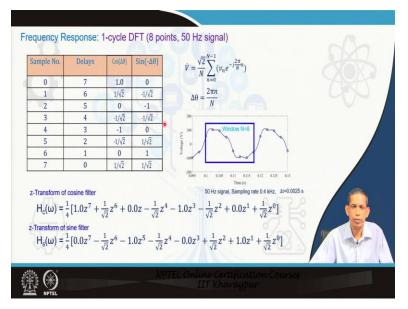
We will see that how we can evaluate the frequency response of different phasor estimation techniques which we have discussed. First let us consider for 1 cycle DFT widely used in relaying principles. So, same 50 Hz signal, 400 Hz sampling means 1 cycle corresponds to 8 points, we will be discussing again for understanding of the concept.
