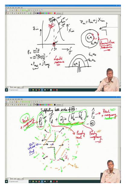
So, we told you that this matching problem is something like this and let us say so, this is the resonant frequency, this is the  $X_{in}$  and this is the  $R_{in}$  with  $Z_{in}$  equal to  $Z_{in} = R_{in} + jX_{in}$ , this is the resonance of the system, typically the resonance of any system, let us say if it is a spherical like a multi-layer sphere resonance of this, so this is epsilon 1 mu 1, epsilon 2 mu 2.
