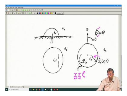
In fact, we can we can work with even a single layer. We can take a single layer of antenna epsilon naught and we have a single layer by image theory we replace the ground plane, so this is my ground plane which is theoretically infinite in extent by image theory we replace the ground plane then have the probe and this is epsilon 0.
