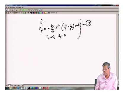
And that eventually works out to be Ephi with Er to be 0 and E theta to be 0. So, therefore the radiated electric field will only have a phi component with the radial component of the electric field 0 and with the elevation component or the theta component of the electric field also to be equal to 0. So we can club all of them into equation 15. So, let us stop here, we will next calculate the radiated magnetic field components by the magnetic current source. Thank you.
