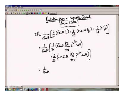
So, last time we had derived the electric field components for the magnetic current source, so now we are going to derive the magnetic field components. So, for derivation of the magnetic field components, we will be needing two operations, one is divergence of  $\mathbf{F}$ , and another is gradient of divergence of  $\mathbf{F}$ . So, let us compute the divergence of  $\mathbf{F}$ .
