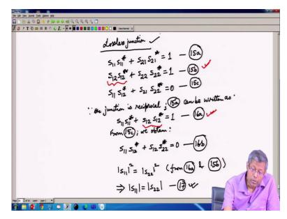
If in addition the junction is lossless, we will have three independent parameters. How? Let us see. So, for the lossless junction we can invoke the conditions and we can apply them for the 2 port network and let us see where we come to after we apply those conditions.
