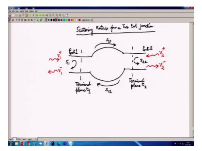
So, consider a two port network. We now specialize from the input network to the two port network. So, consider a two port network. Here it is  $S_{21}$ ,  $S_{12}$ . So, this is the general depiction of the two port network. So, what do we have?
