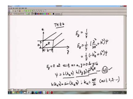
The waveguide is bounded by conducting walls on all four sides so, this is the waveguide let us called this direction x, this direction y, so this direction will be z and let this dimension be a, and let that dimension be b. If we would look at the z component of the electric field, for the TM to z mode does not have Hz component.
