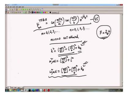
So therefore the Psi function for mn<sup>th</sup> mode corresponding to the transverse electric to z field
