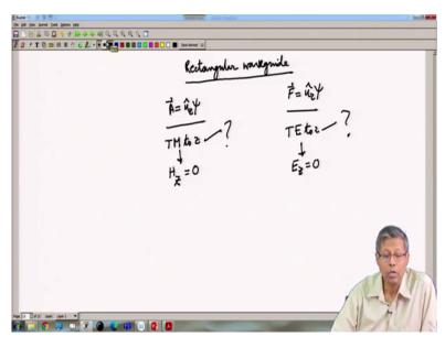
We had previously constructed the electromagnetic field solutions for two cases, one when the magnetic vector potential was **A** equal to **uz** Psi, and another when the electric vector potential was **F** is equal to **uz** Psi, these are the two cases for which we had constructed the, the field solutions. And we found that for this case where the magnetic vector potential was **z** - directed it gave rise to a transverse magnetic to z mode that is the mode for which Hz equal to 0.
