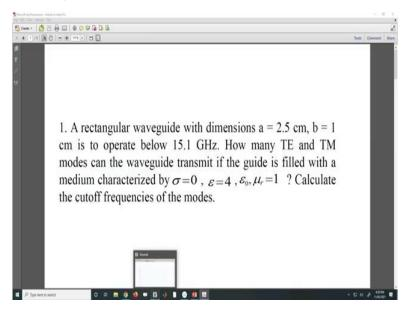
Hello everyone, today we will solve numerical problems based on Rectangular Waveguide. So, our first problem states that, a rectangular waveguide with dimension a equals to 2.5 centimeter, b equals 1 centimeter is to operate below 15.1 Gig Hertz. How many TE and TM modes can the waveguide transmit if the guide is filled with a medium characterize by sigma equals to 0, Epsilon equals to 4, Epsilon Naught and Mu are equals to 1. Calculate the cut-off frequencies of the modes.
