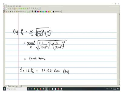
So, in the given question, there is 1 centimeter cross 3-centimeter rectangular air-filled waveguide, and it is operating in TE 12 mode.
