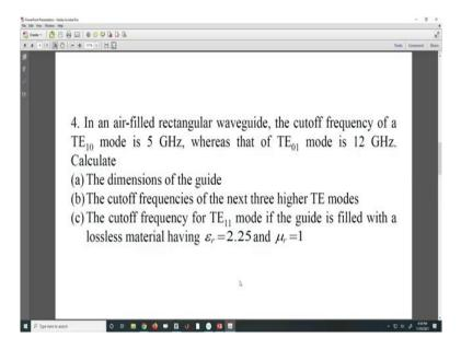
4. In an air-filled rectangular waveguide, the cutoff frequency of a  $TE_{10}$  mode is 5 GHz, whereas that of  $TE_{01}$  mode is 12 GHz. Calculate
