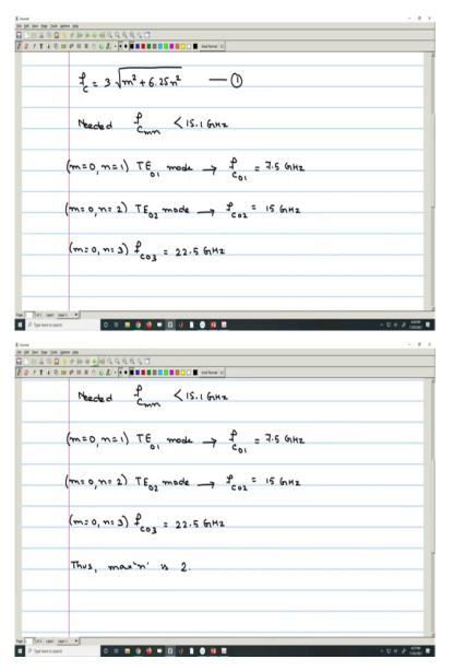
here it is given that, we need to operate the waveguide below 15.1 Giga Hertz. So, it is needed to be that fc mn should be less than 15.1 Gig Hertz. Now, a systematic way of doing this is to fix m or n and then increase the other until fc mn is greater than 15.1 Giga Hertz.
