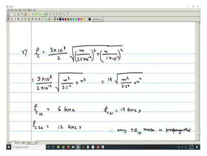
So, a microwave transmitter is connected by an air-filled waveguide, of cross section 2.5 centimeter cross 1 centimeter. So, again we will start with calculating the cut-off frequency
