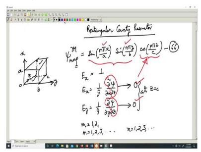
So, the first thing we want to understand about the rectangular cavity resonator is, derivation of the modes in the rectangular cavity resonator. We did the same thing for the rectangular waveguide, we first of all found out the potential functions for the rectangular waveguide. And from the potential functions we found out the, the field distributions of the TE to z and the TM to z mode sets in the rectangular waveguide.
