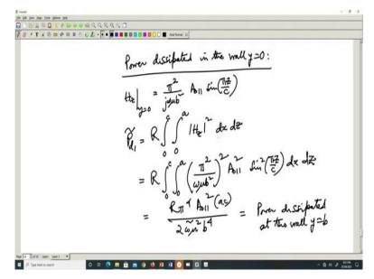
So, now for this structure power dissipated in the wall y equal to 0, we find that the only tangential component of the magnetic field, which is, which is present at y equal to 0.
